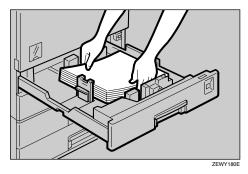
While pressing the release lever, adjust the side guides to the new paper size.
